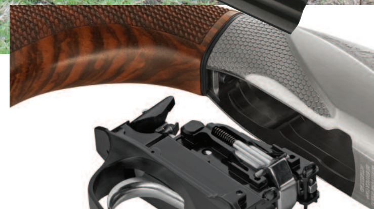
The Benelli 828U features a removable trigger mechanism – handy for cleaning. This gun has strikers rather than hammers.
